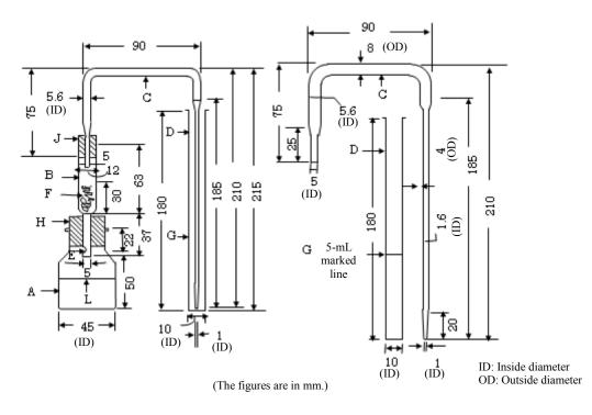
Figure Arsenic limit test apparatus
