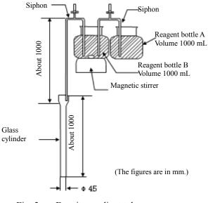
Fig. 3 Density gradient tube
