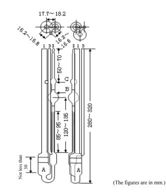
Fig. 1 Capillary tube viscometer
