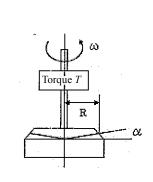
Fig. 3 Single cylinder-type rotational viscometer
