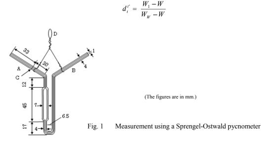
Further, when measurements for a sample solution and water are performed at the same temperature ( $t^{\circ}C = t^{\circ}C$ ), the density of the sample solution at the temperature  $t^{\circ}C(\rho_T^{t'})$  can be calculated from the measured specific gravity  $d_t^{t'}$  and the density of water at the temperature  $t^{\circ}C(\rho_W^t)$  indicated in Table 1 by using the following equation.
